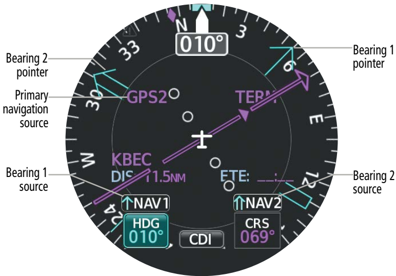
'HSI' Page with Bearing Pointers
