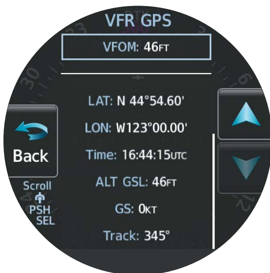
VFR GPS Current Location
